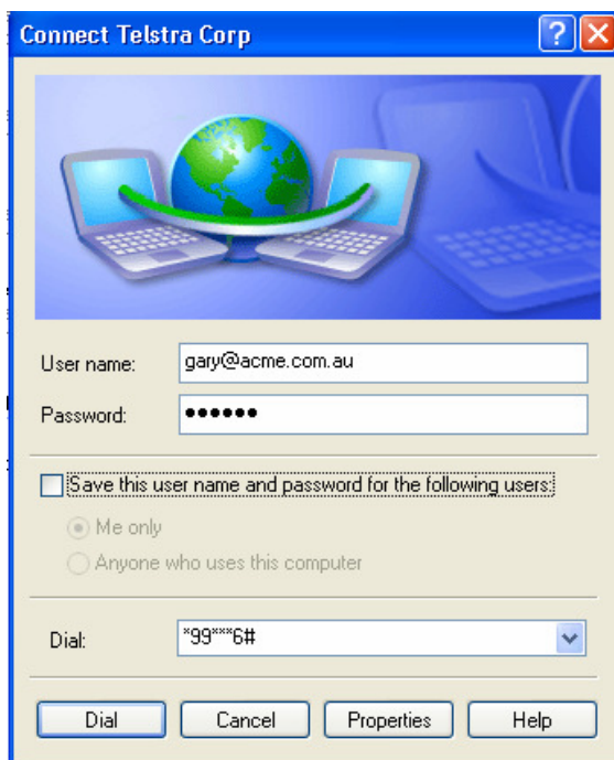
Figure 17: Showing Dial Up Network window populated with username password and dial number to connect using Context ID = 6.
